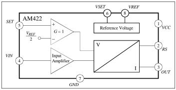
Figure 1: block diagram of the voltage-to-current transmitter AM422
