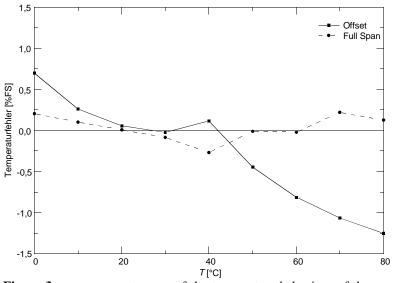
Figure 3: measurement curves of the temperature behaviour of the entire system
